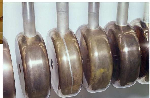
*LINAC2 (top) and LINAC2 drift tubes (right)*
