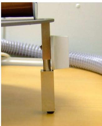
Fig. 3: Turning knob to tilt gyroscopic table
